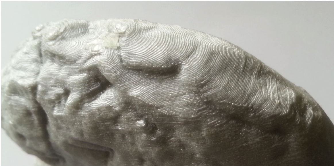
Figure 5 A technological mediation artefact: print layers visible as topographic contours at an ‘end’ of the FDM print.
