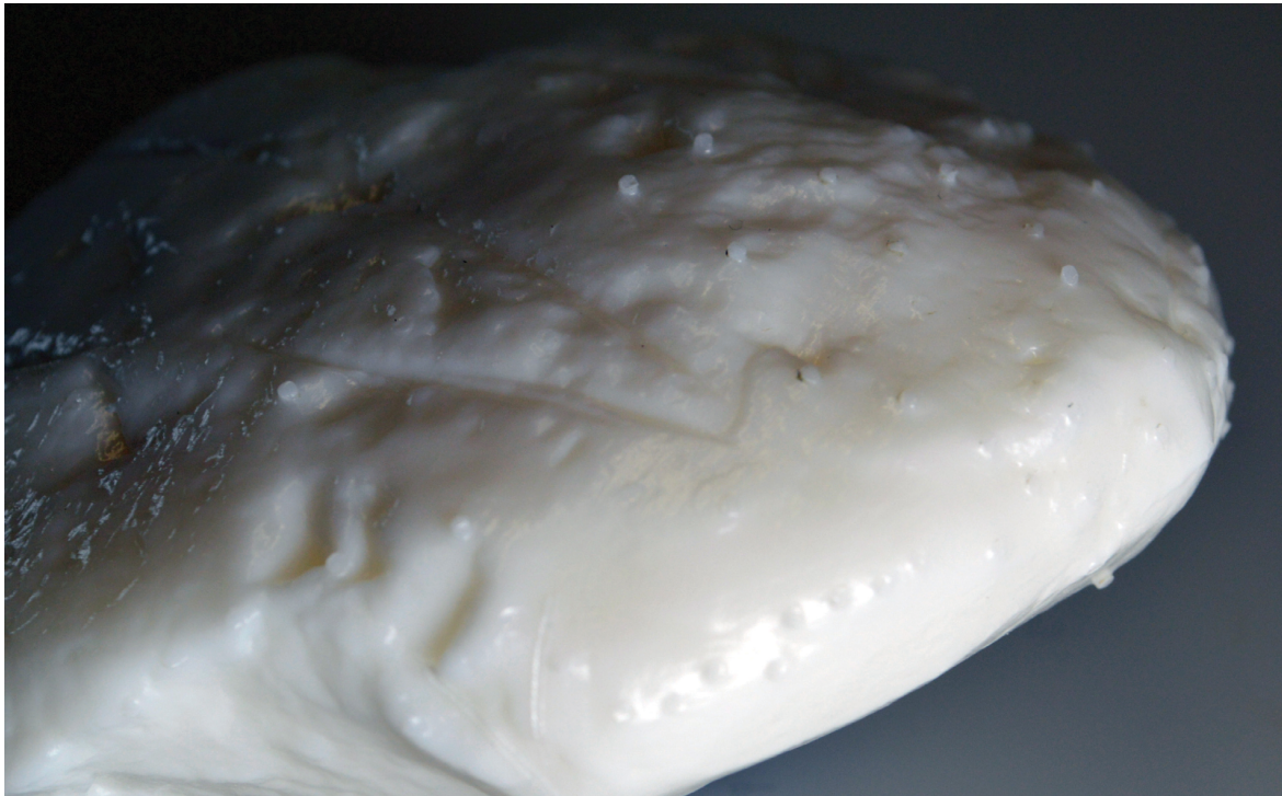
Figure 2 Reverse of the SL resin print with bumps left after breaking the scaffold away.
