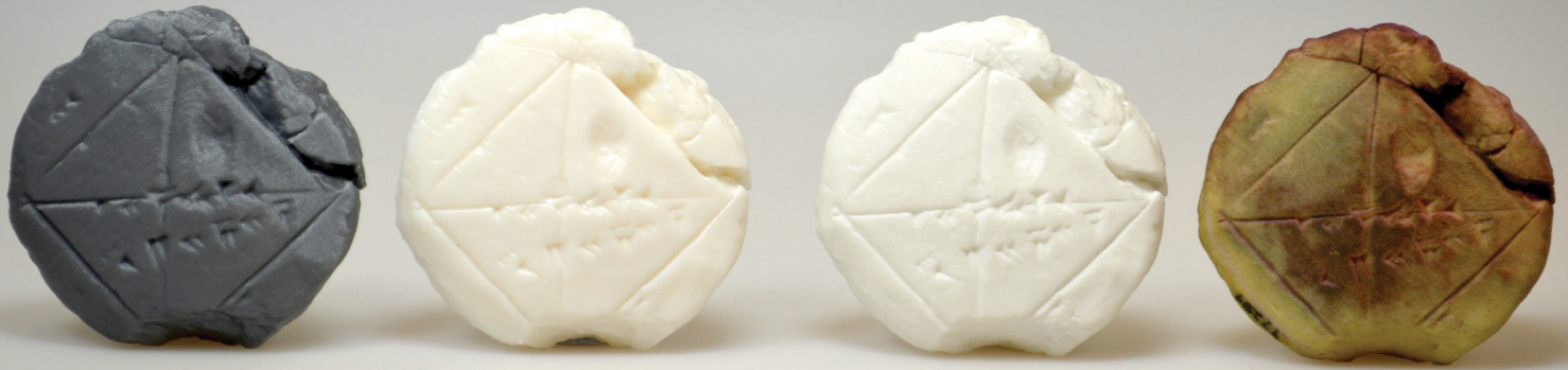
Figure 3 Left to right: fused-deposition PLA print; stereolithographic resin print; laser-sintered nylon print; gypsum print.
